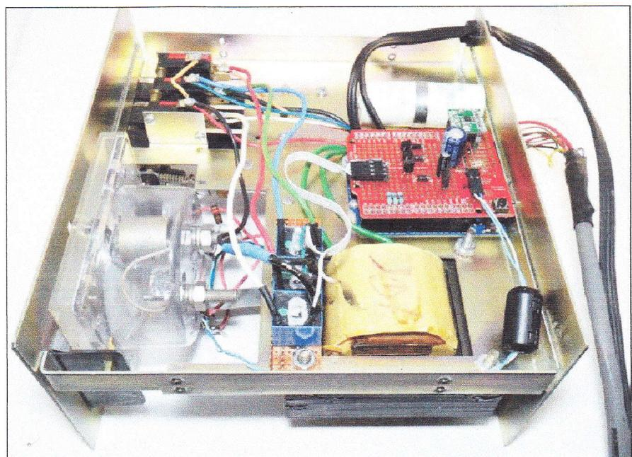
Figure 2 — Modified Ham III rotator controller.
