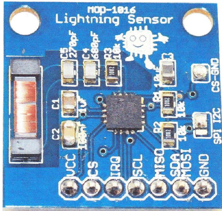
Figure 1 — Lightning sensor module from Embedded Adventures.
