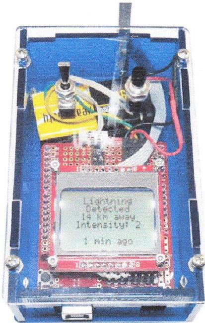
Figure 3 — Arduino-powered lightning detector.
