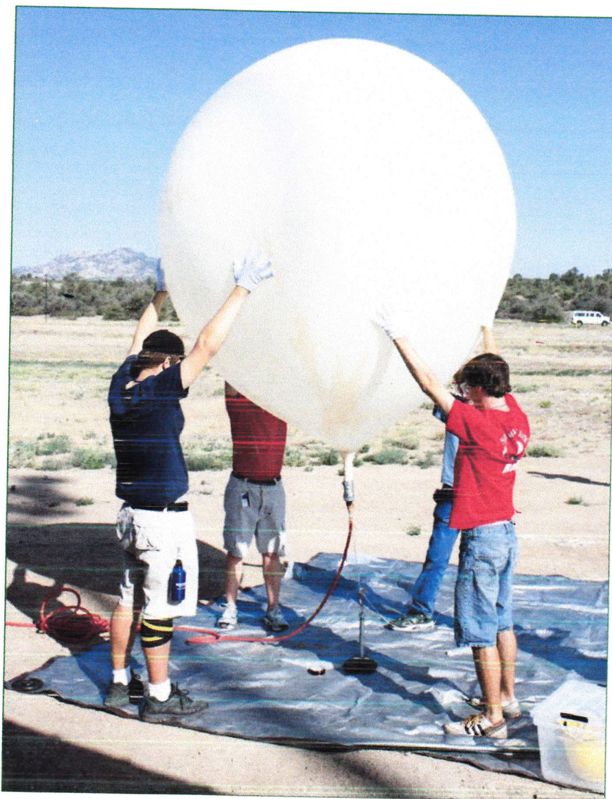
Figure 1 — Students participating in a summer camp at Embry-Riddle Aeronautical University steady a high-altitude balloon before launch. The balloon reached 85,000 feet while carrying an APRS tracker and sensor package.
