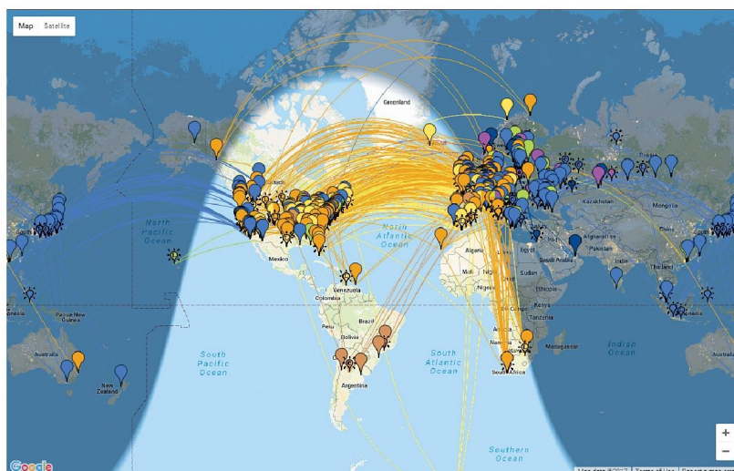
Figure 2 — PSK Reporter world map showing open propagation paths for spotted JT65 and JT9 signals over a 1-hour interval around 1630 UTC on February 13, 2017. Different colors indicate signals on different bands. Magenta is 80 meters, blue is 40 meters, yellow is 20 meters, and brown is 15 meters.
