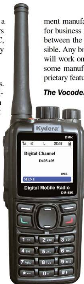
Figure 1 — A DMR handheld transceiver can have no display, a monochrome display, or a color display like this Kydera model. [Image courtesy of Kydera]
